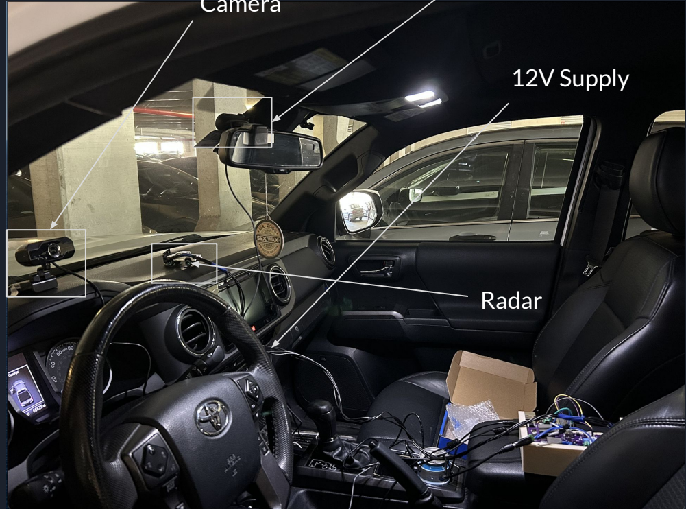
Traffic Facing Camera
